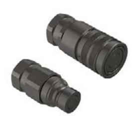
Flat face Male and Female couplings. The flat valve shut-off system prevents contamination and spillage. Real maximum working pressure of 35 MPa and Zinc-Nickel plating. Available sizes: 1/8", 1/4", 3/8", 1/2", 5/8", 3/4", 1". Interchangeable according to ISO 16028. Size 1/8" has surface treatment in Mate 500 (CrIII) and it is not ISO interchangeable.
