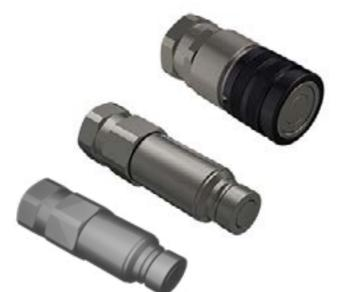
Flat face Male and Female couplings. The flat valve shut-off system prevents contamination and spillage. Real maximum working pressure of 35 MPa and Zinc-Nickel plating. Connectable under residual pressure. It is possible to couple either a 3FFH Female half under pressure with a FFH Male half, or a 3FFH Male half under pressure with a FFH Female half. Available sizes: 3/8", 1/2", 5/8", 3/4". Interchangeable according to ISO 16028.
