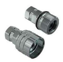
Screw-to-Connect Male and Female couplings, suitable for general purpose applications. High resistance to pressure and flow impulses. Connectable under residual pressure. Available sizes: 1/4", 3/8", 1/2", 3/4", 1", 1-1/2". Interchangeable according to ISO 14541 standard only for sizes 1/4", 3/8", 1/2", 3/4".
